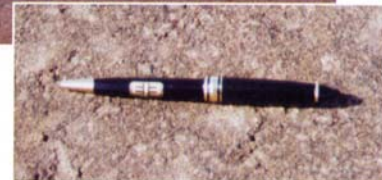
The 6-inch-deep recycled asphalt base (foreground) is topped off with a hot-mix asphalt wearing surface at a compacted depth of 2 inches. Inset: this smooth base surface is the product, in part, of a homogenous mix that began with recycled material with a gradation of 2-inch minus.
